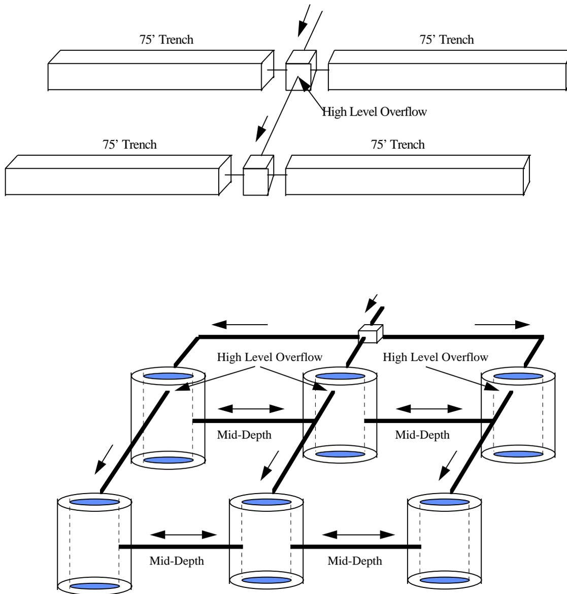
Figure 10-6 - Combination Level and Serial Distribution
