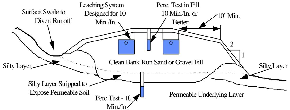
Figure 17-5 - Soil Replacement Filling
