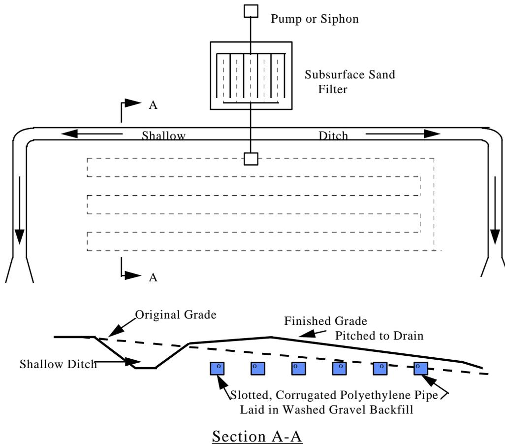
Figure 13-2 - Subsurface Irrigation System
