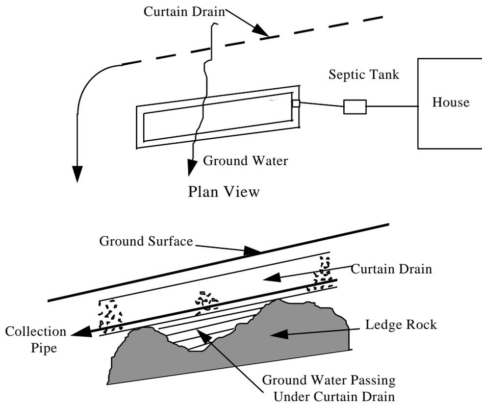
Figure 15-1 - Profile Through Curtain Drain
