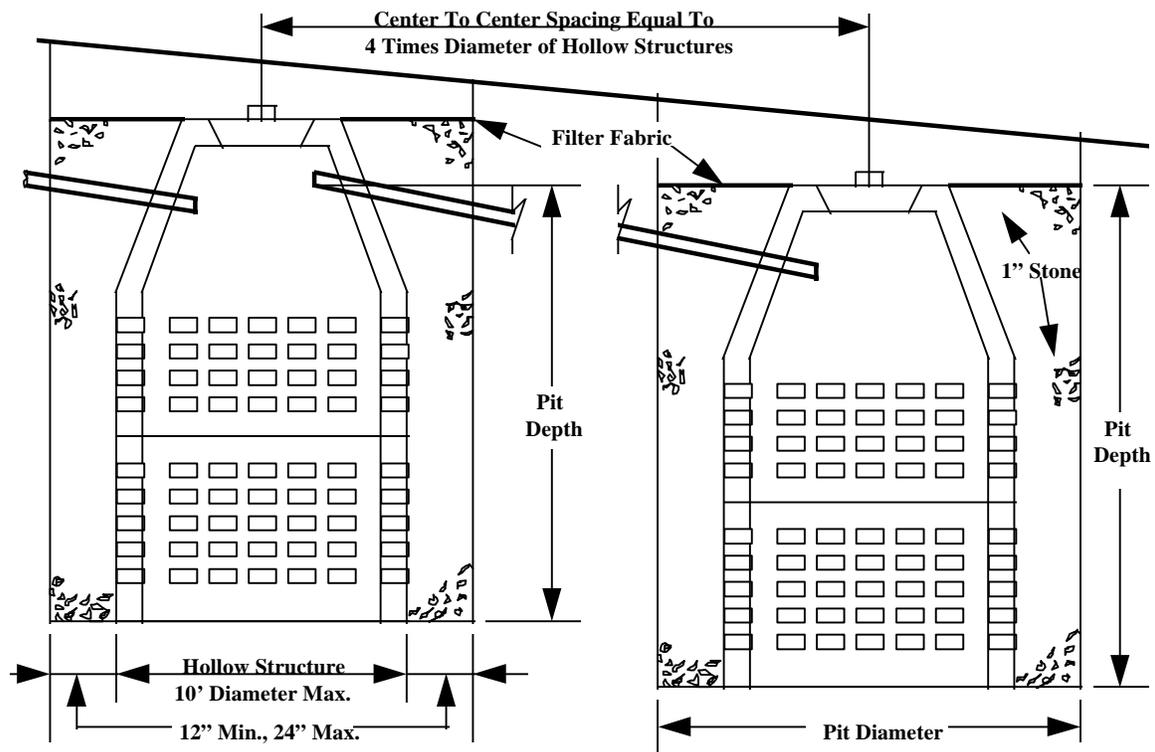
Figure 10-5 Pits at Different Elevations - High Level Overflow
