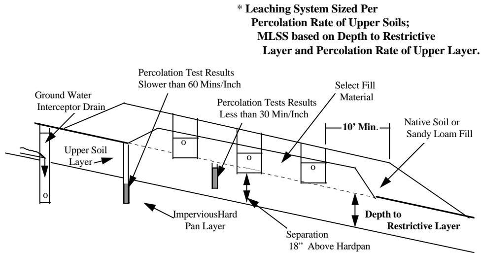
**Figure 16-3 - Impervious Hardpan**
