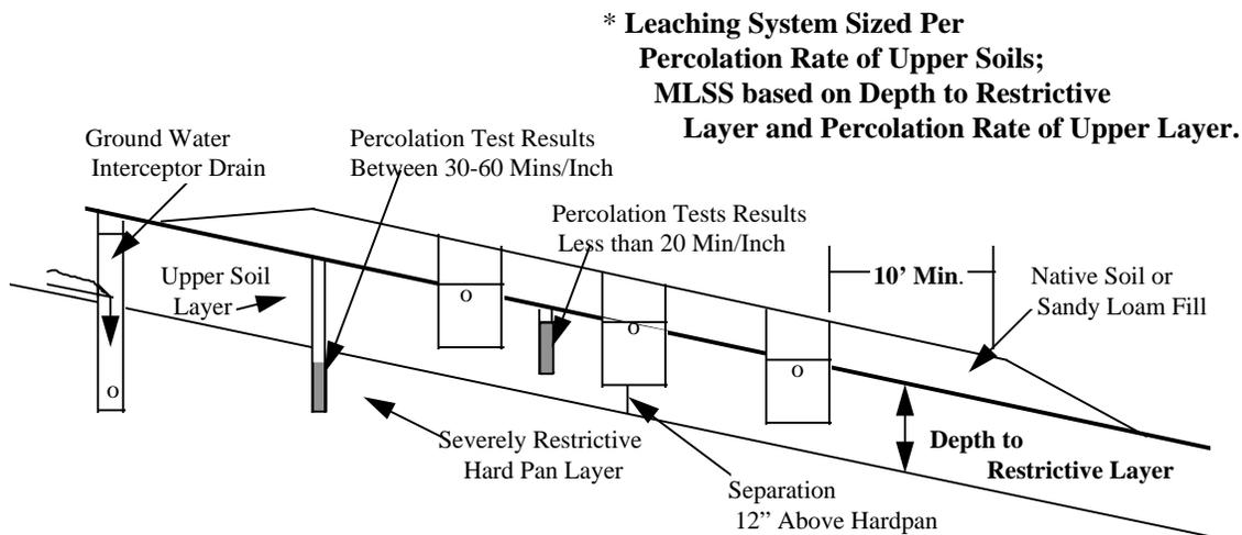
Figure 16-2 - Severely Restrictive Hardpan
