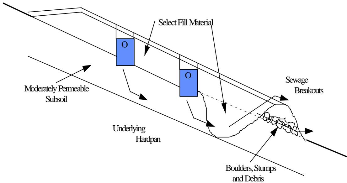
Figure 17-6 - “Keyed-In” Cut In Downslope Subsoil
