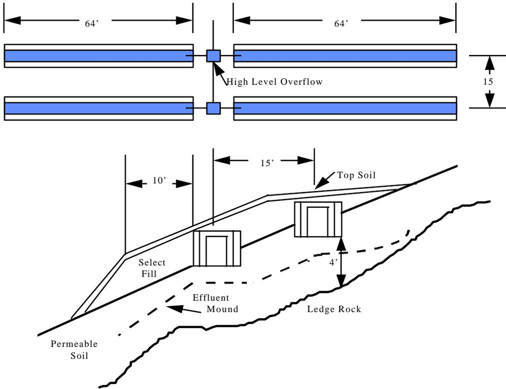
Figure 25-3 - Galleries Spread On Slope Over Ledge Rock
