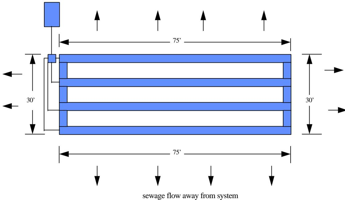
Figure 25-4 - Flat Lot System with Radial Flow
