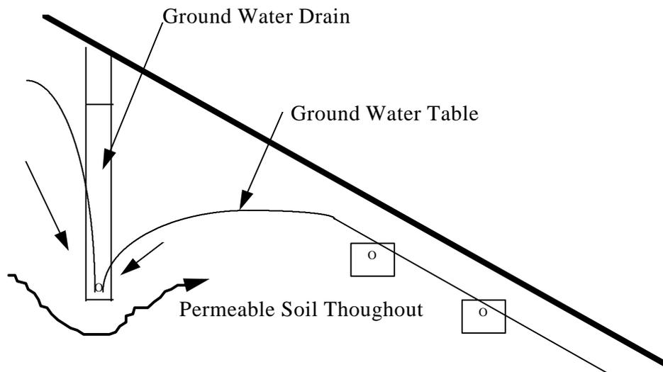
**Figure 7-3 - Ground Water Drain on Permeable Slope**
