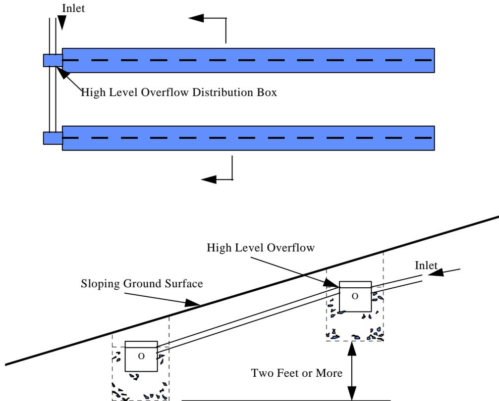
Figure 10-3 - Serial Leaching Trenches
