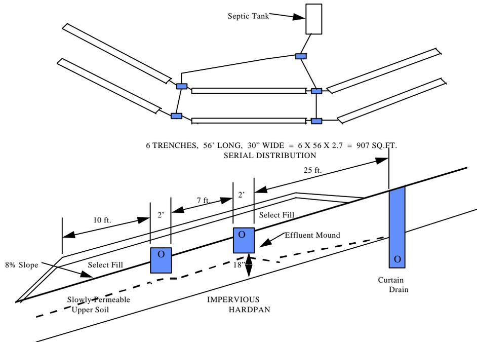
Figure 25-2 - Trenches In Slowly Permeable Soil Spread On Slope
