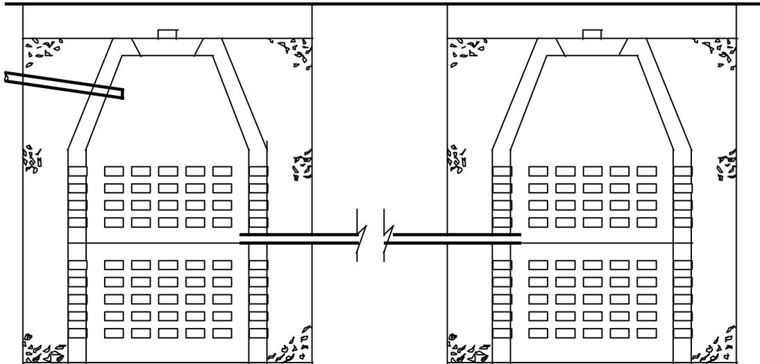
Figure 10 -2 - Pits at Same Elevation - Connection at Mid-Depth
