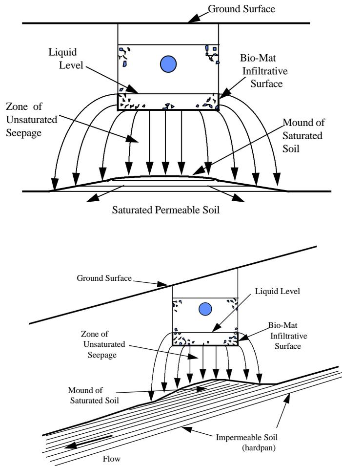
**Figure 11-1 - Effluent Mounding**
