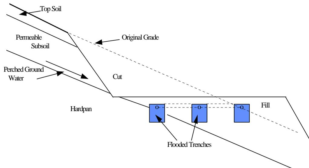
Figure 17-4 - Cut and Fill on Slope
