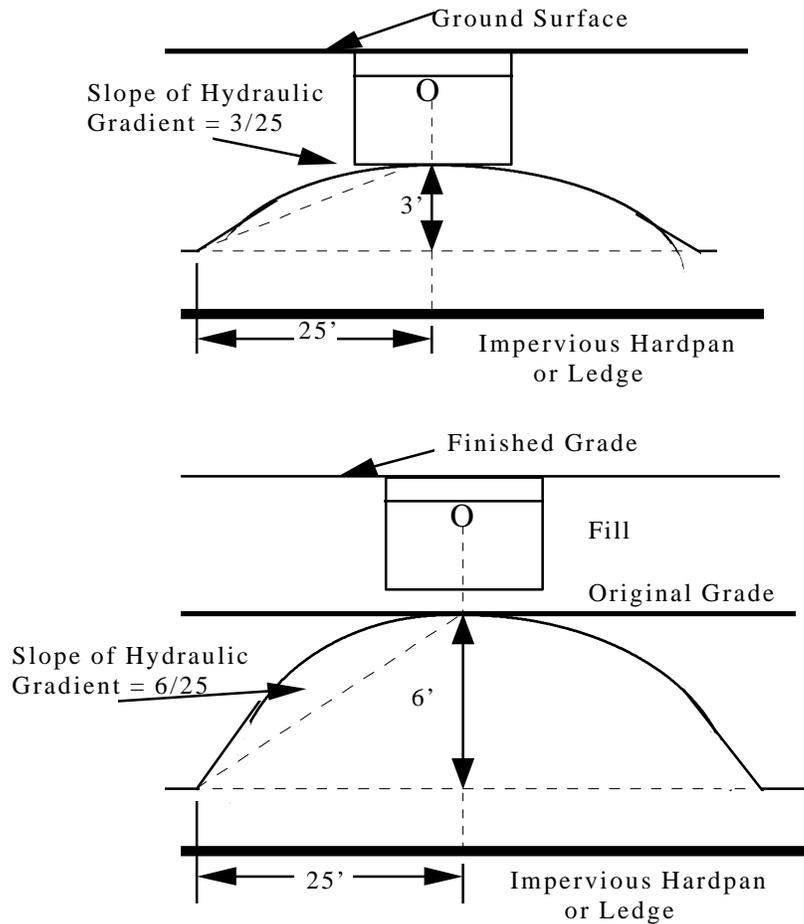
Figure 11-3- Elevating Trenches to Increase Hydraulic Gradient
