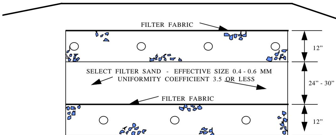
Figure 33-1 Subsurface Sand Filter
