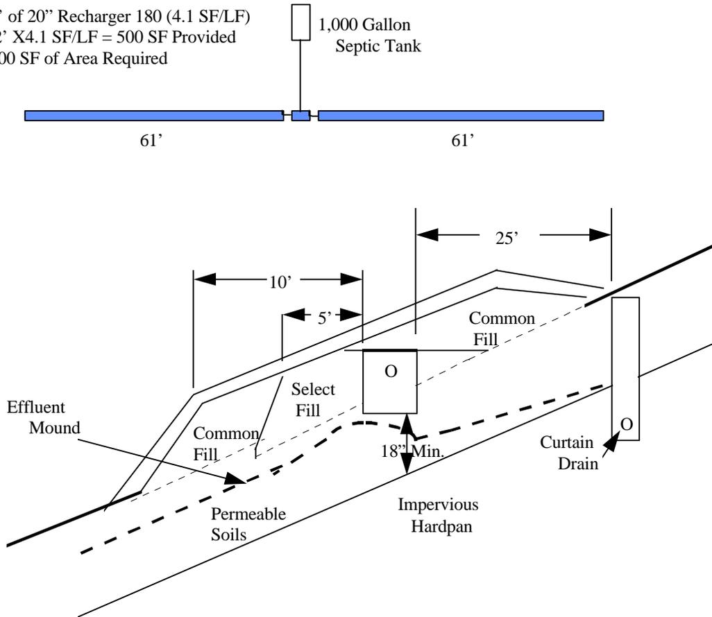
Figure 25-1 - Trenches Spread On Slope Over Impervious Hardpan
