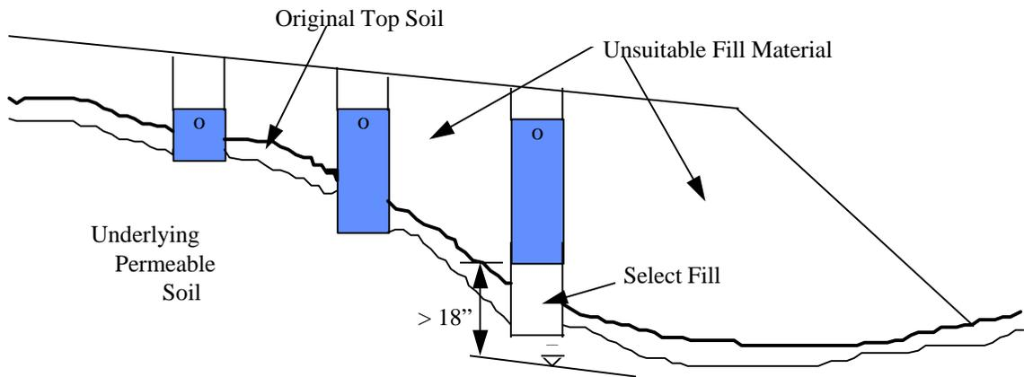
Figure 17-2 - Leaching System In Unsuitable Fill
