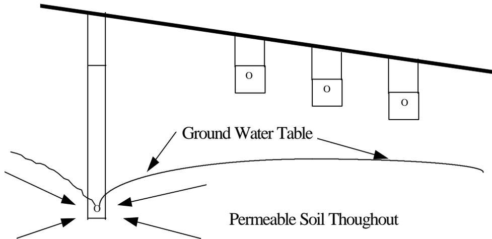
**Figure 7-2 - Ground Water Drain In Permeable Soil**
