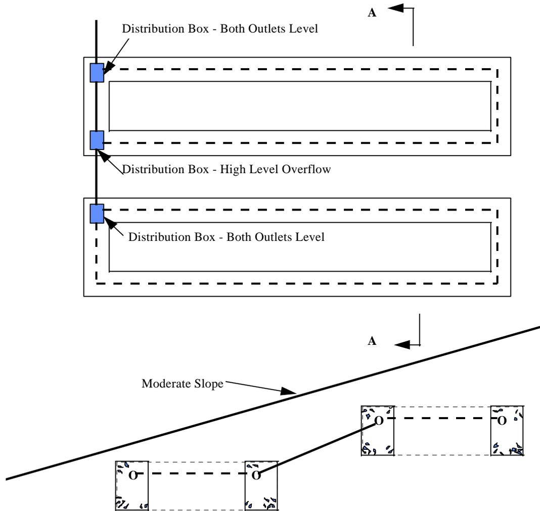
Figure 10-7 - Two Level Trench Systems in Series
