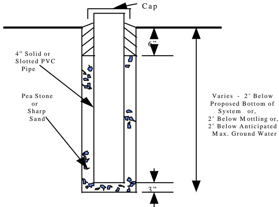
Figure 6.1 Ground Water Monitoring Well
