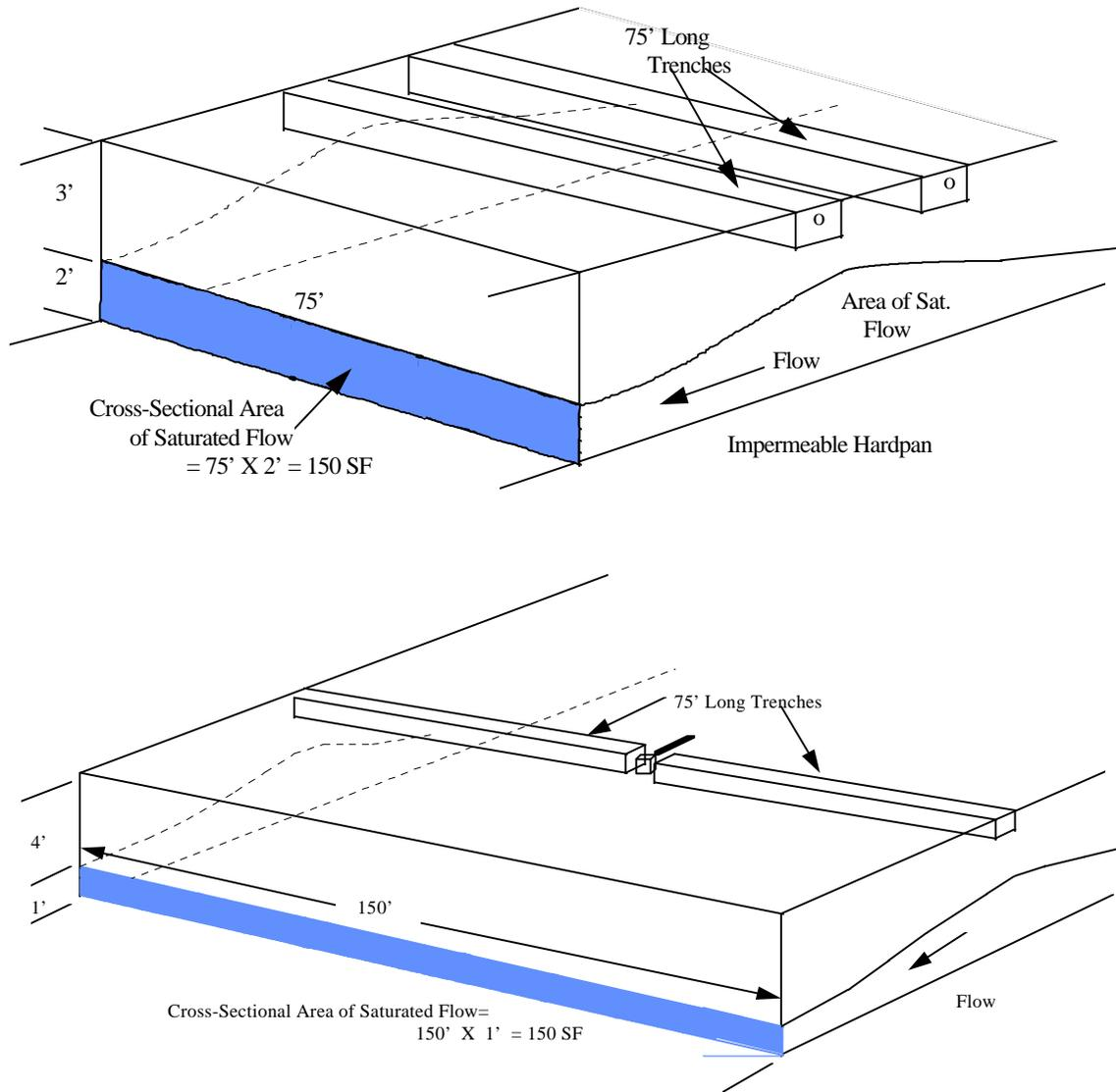
**Figure 11-2** Spreading Trenches to Reduce Effluent Mounding
