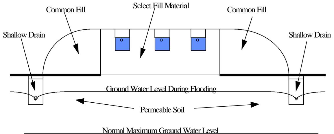
**Figure 7-4 - Shallow Drains To Control Flooding**
