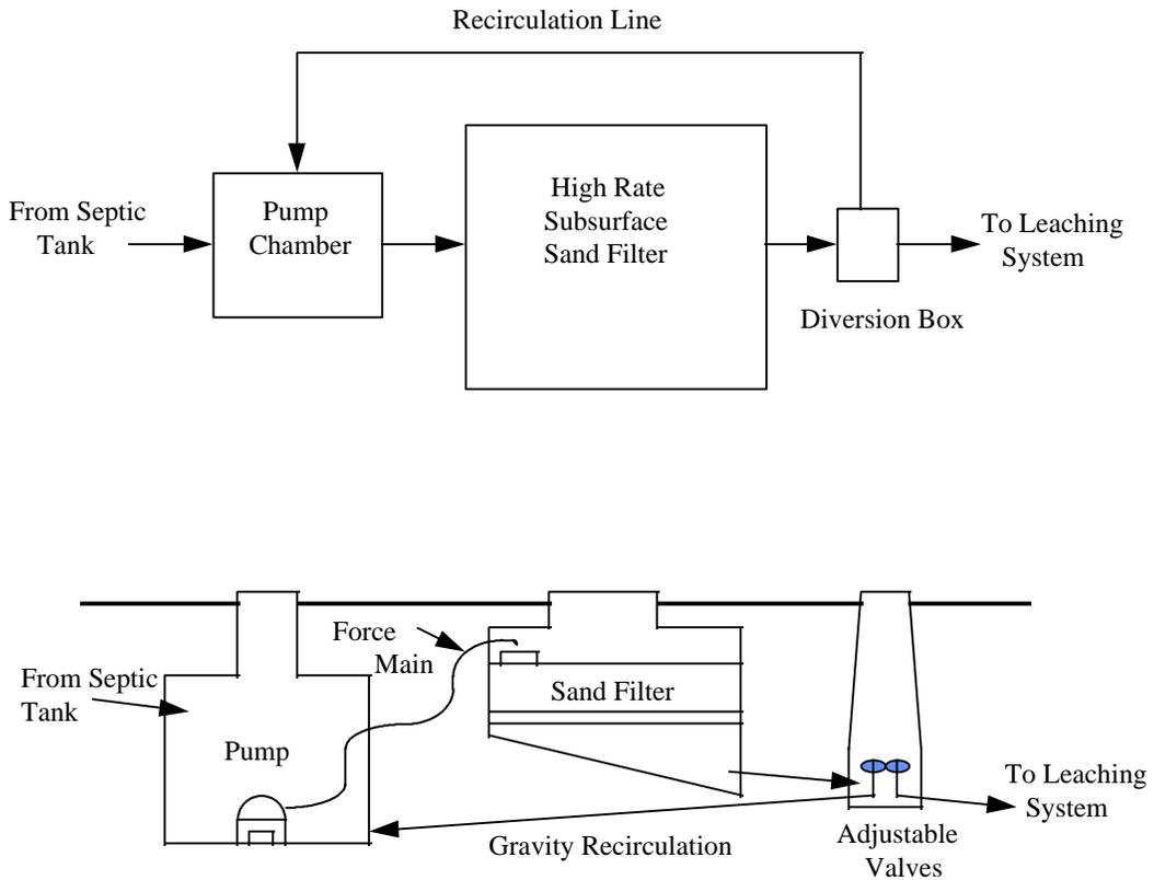
Figure 33-3 Recirculating Sand Filter
